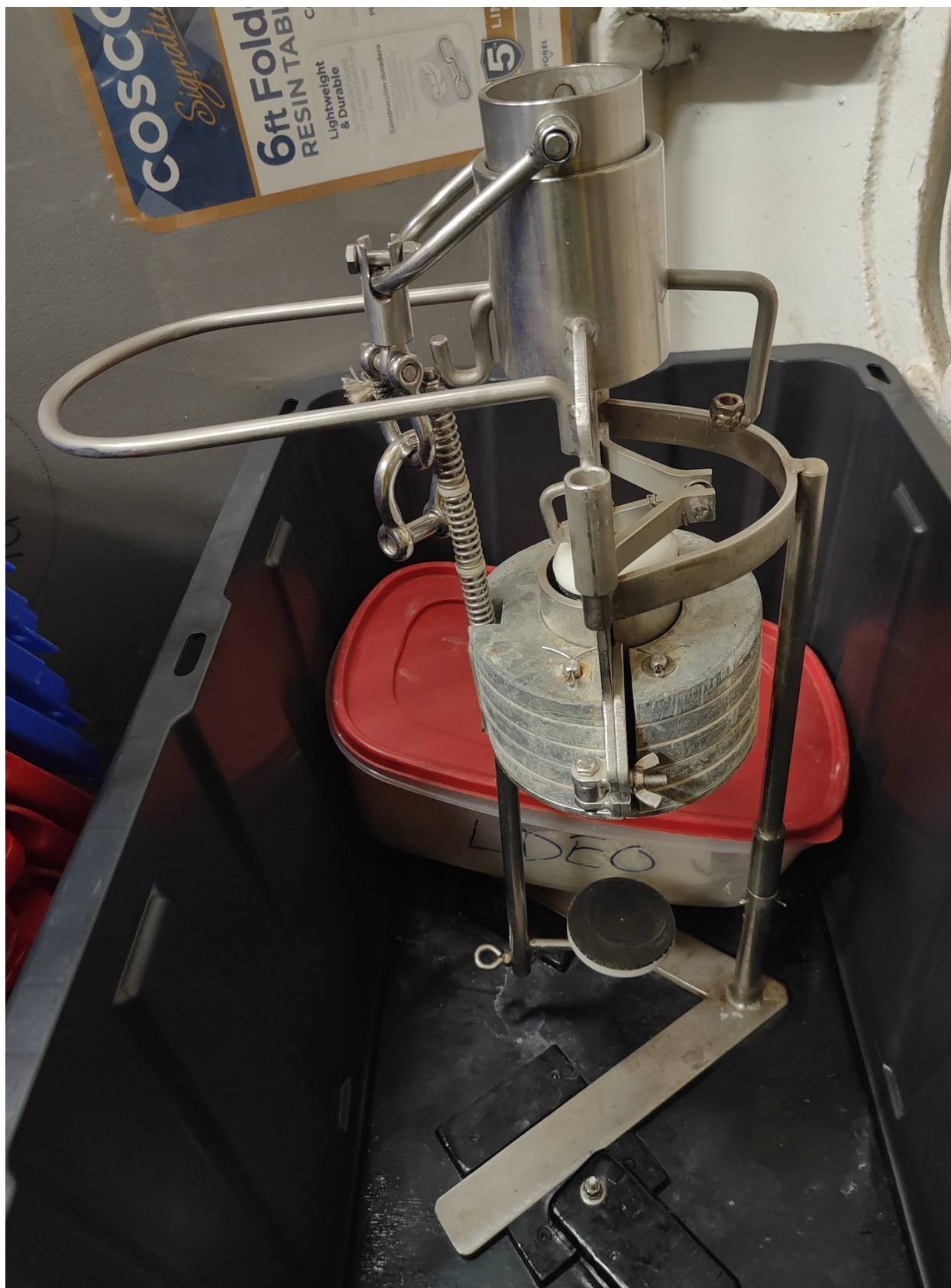
Fig. 12: Monocore, for hanging below the ODF rosette.
