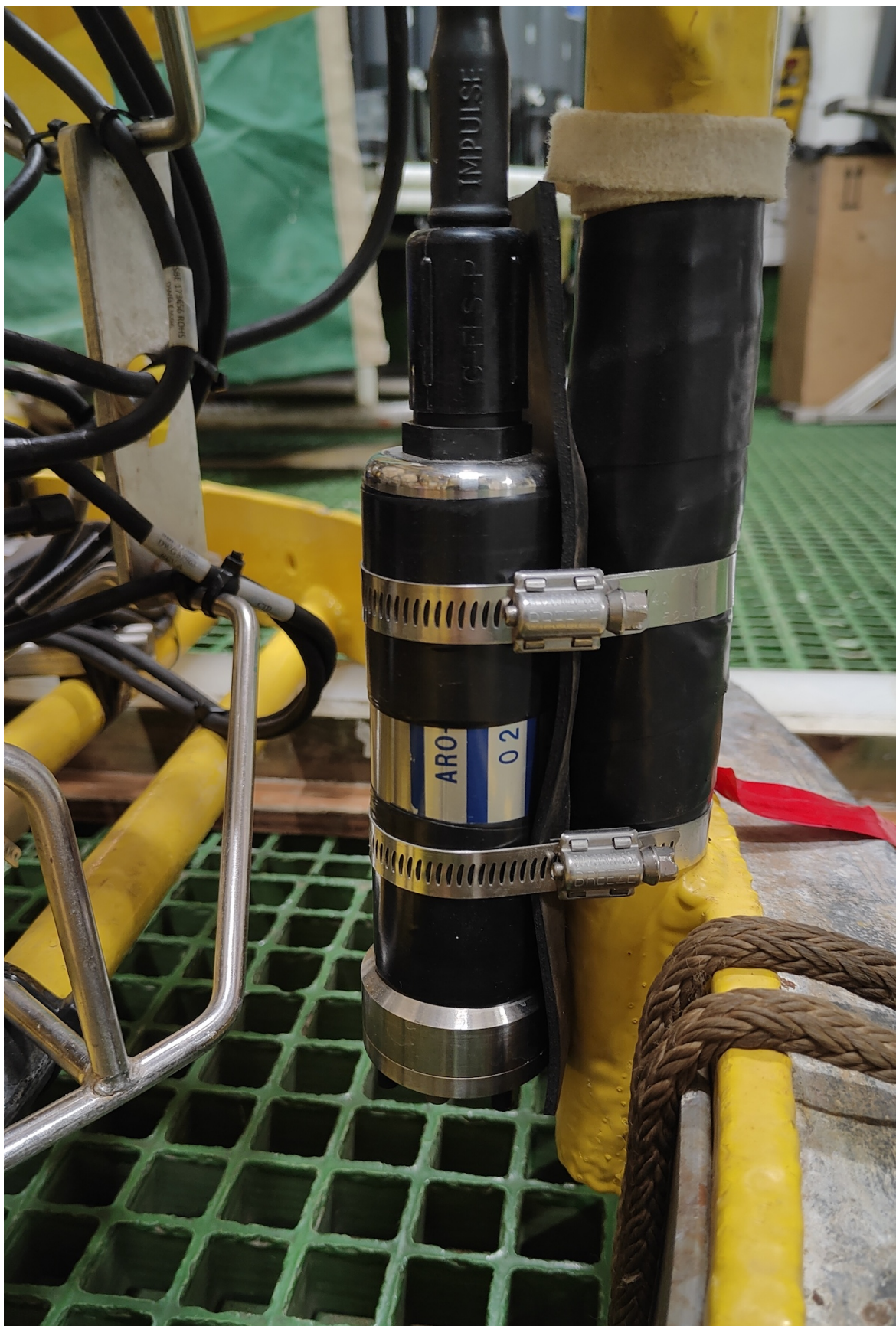
Fig. 8: ODF RINKO sensor mounting position, away from the WHOI UVP .
