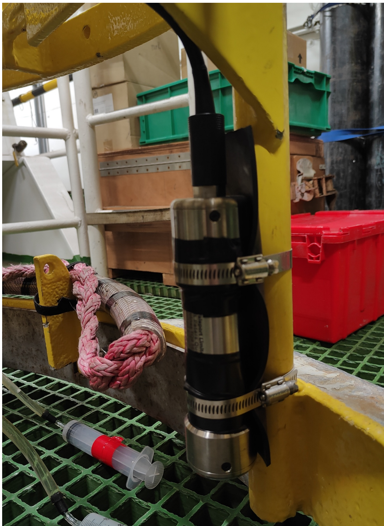
Fig. 6: ODF altimeter mounting position.
