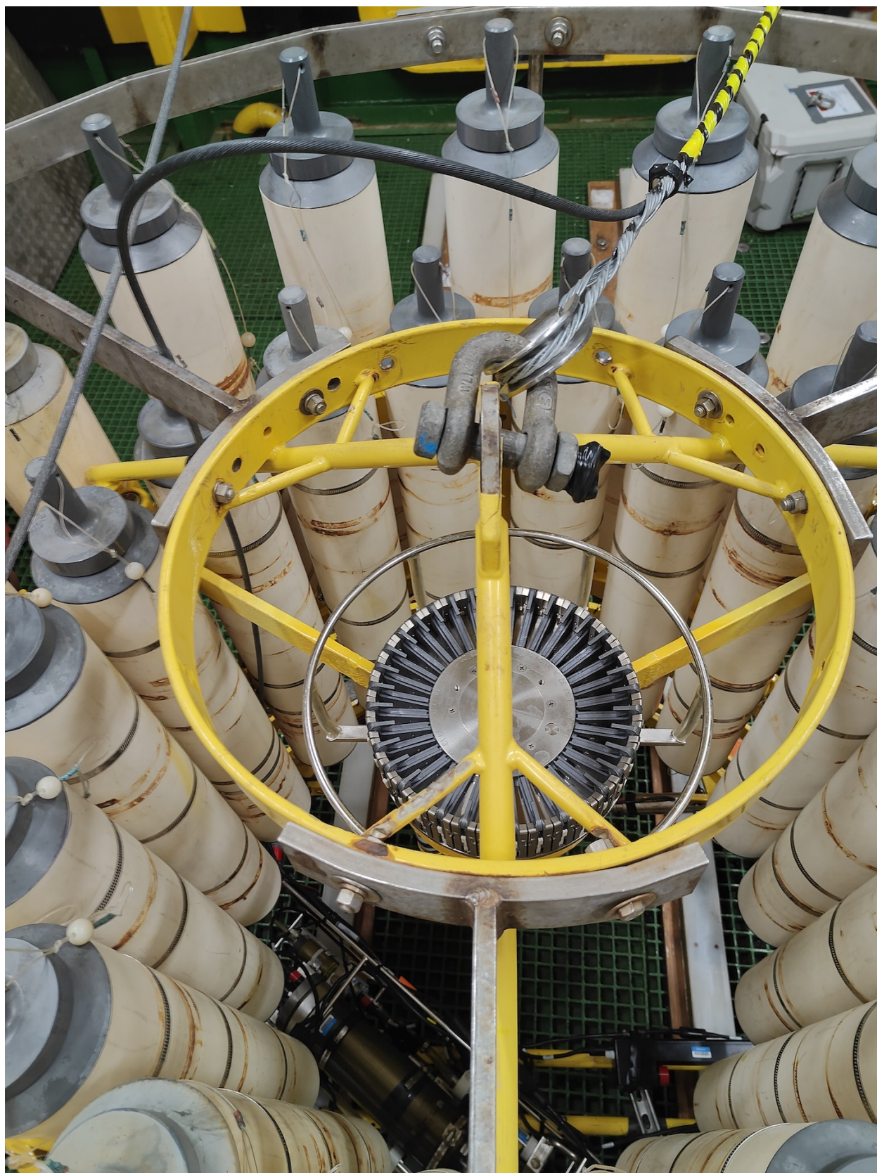
Fig. 4: Package sensor setup, seen from above.
