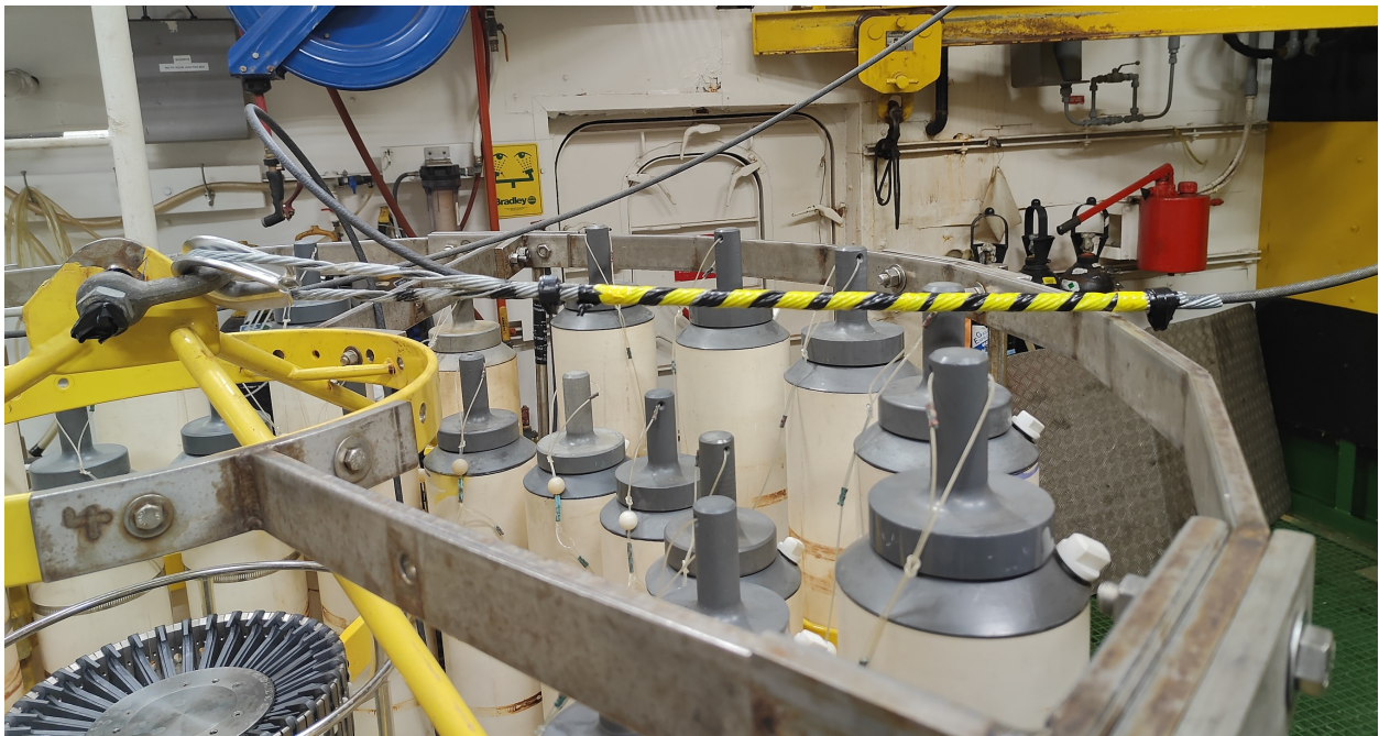
Fig. 10: Guy grip primary termination, located above the rosette package.
