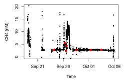
Figure 4.14-2. Comparison of discretely collected surface samples from the <5 m Niskin bottle (red dots) to underway system measurements.
